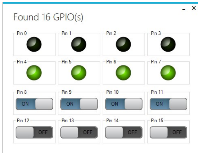
Figure 9: The status changed by connect DOs to DIs in Dry Contact configuration.
